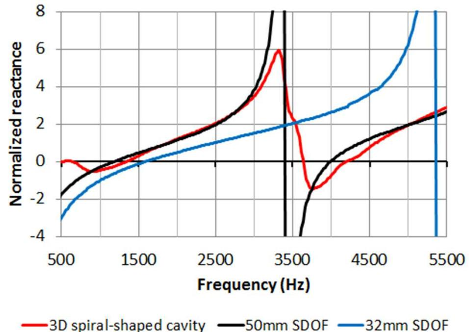
Equivalent acoustic length is increased by more than 50%
