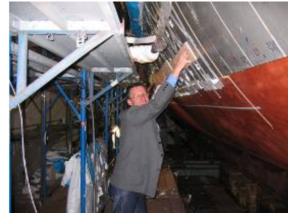
Acoustic coating on a modern submarine
