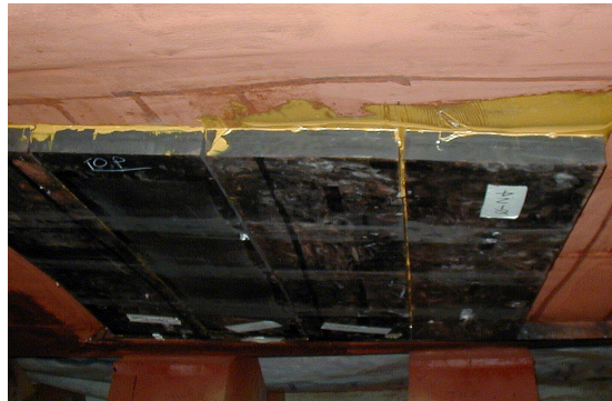
Experimental decoupling coating on a surface ship
