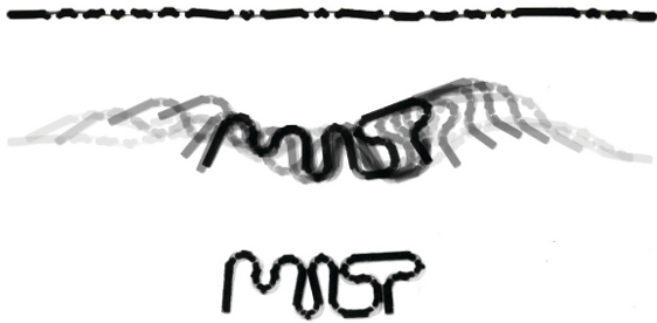
A sequence of images demonstrating the self-folding of a 4D printed multi-material single strand into the world of MIT
